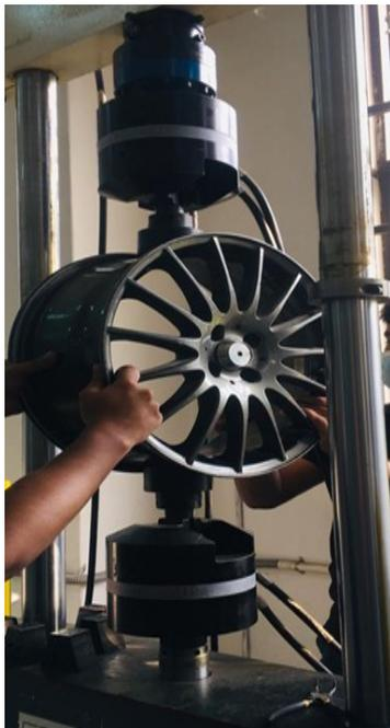
Figure 10. Compression test of the rim using UTM
